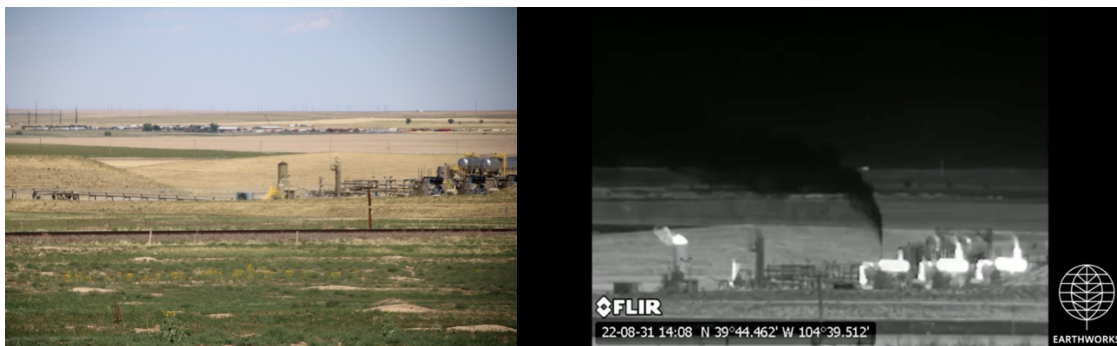
Figure 1: (Left) Photo of an oil and gas midstream facility located .8 miles from the Aetna Estates mobile home community in Arapahoe County. (Right) OGI image of the same facility from the same vantage point showing a plume of uncontrolled hydrocarbon emissions from a blowdown of one of the compressor engines.
