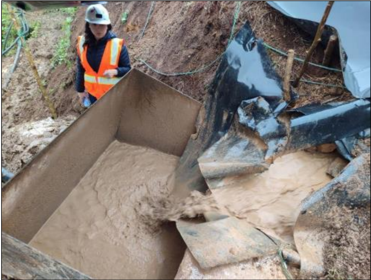
Figure 18. The water and tailings that were discharged from Pond No. 15 were collected in a metal container and then transferred to Pond No. 9 (see Fig. 4). Photo from Municipio de Cotacachi (2023a).
