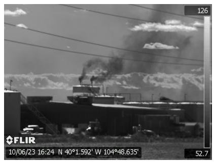
OGI image highlighting uncontrolled hydrocarbon emissions from produced water storage tanks on a produced water storage and disposal facility located in a DIC<sup>16</sup> and adjacent to the New Vision mobile home community. These emissions are not in violation of APCD regulations
