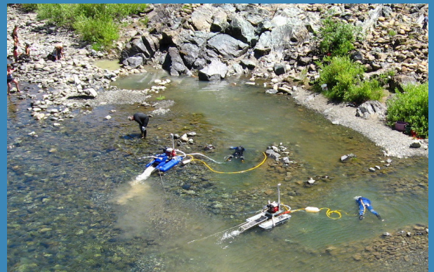
Suction dredge mining in Oregon uses hoses to vacuum up the sediments in search of gold. Suction dredge mining uses placer claims, rather than lode claims. Photo by KS Wild.
