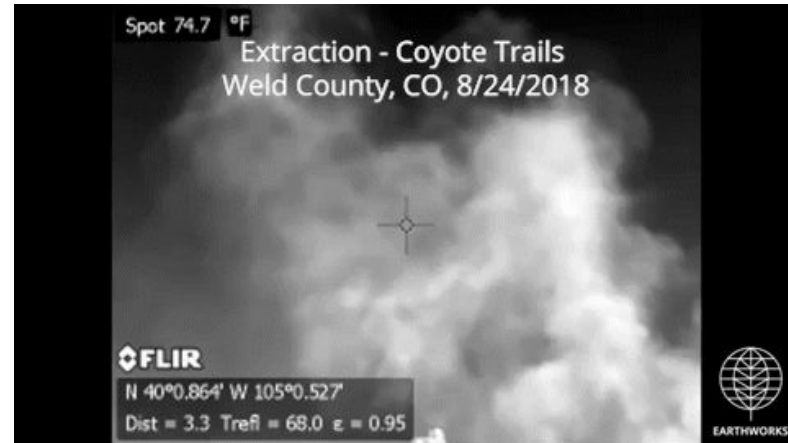
Hydrocarbon emissions from incomplete combustion at well pad during drilling in 2018
