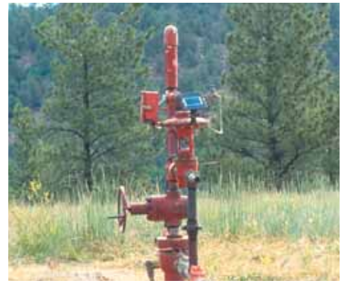
FIGURE I-7. CHRISTMAS TREE The wellhead of a gas well. The first step as natural gas leaves the ground. Photo by OGAP.
