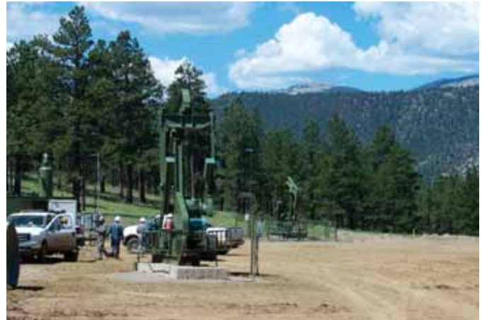
FIGURE I-37. A VERTICAL AND HORIZONTAL WELL DRILLED ON ONE PAD. Photo printed with permission of Vermejo Park Ranch.
