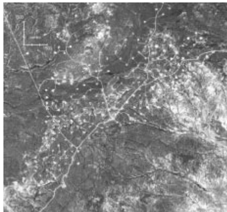
Top: Aerial photography showing gas fields in Wyoming in 1994, prior to major expansion of gas play. Below: Satellite image from 1999 showing the same area at the same scale. New well pads and roads are clearly visible as bright patches and lines; wastewater pits are dark spots on the well pads. This image shows about 97 of the 233 new wells drilled since 1994 in the Jonah project. BLM has already permitted over 6,000 gas well pads or locations in the same vicinity out of 10,000 to 15,000 that are planned for this area in southwestern Wyoming in the next decade.
