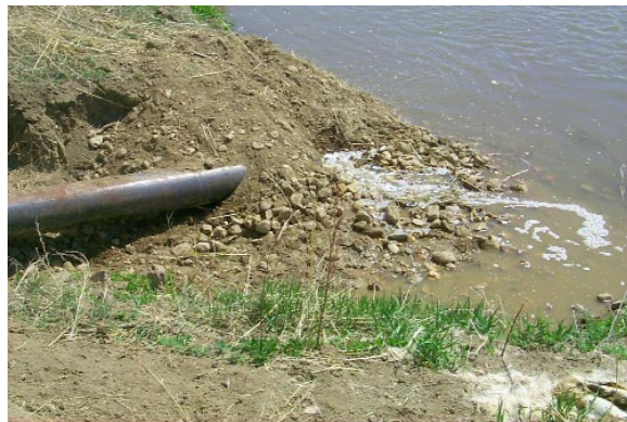
Above three: CBM discharges from one outfall can wreak havoc on the environment, particularly soils and native vegetation.
