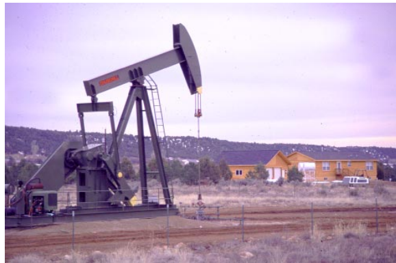
A pump jack is used to pump water to create coalbed methane near a home outside of Durango,. State regulations, which can be waived, generally require drillers to drill wells at least 150 feet from Coloradans’ homes.
