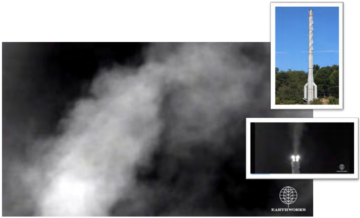
Emissions venting seen with optical gas imaging. Bluestone Gas Processing Plant, Butler County, Pennsylvania. Images by Earthworks.
