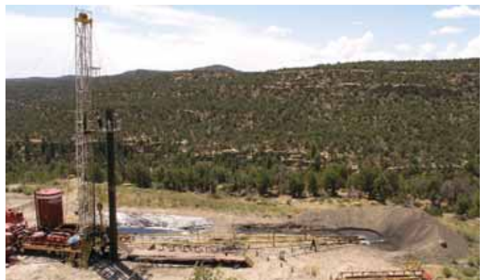
FIGURE I-39. TYPICAL COMPLETION WITH A FLARE BERM AND WASTE PITS. Photo by Dan Randolph
