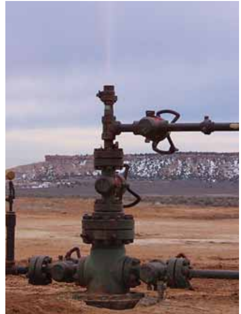
FIGURE I-19. VENTING OF GAS WELL Source of methane, a greenhouse gas.
