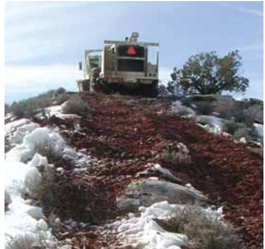
FIGURE I-2. SEISMIC EXPLORATION 30-ton thumper trucks leave lasting impressions on the surface.
