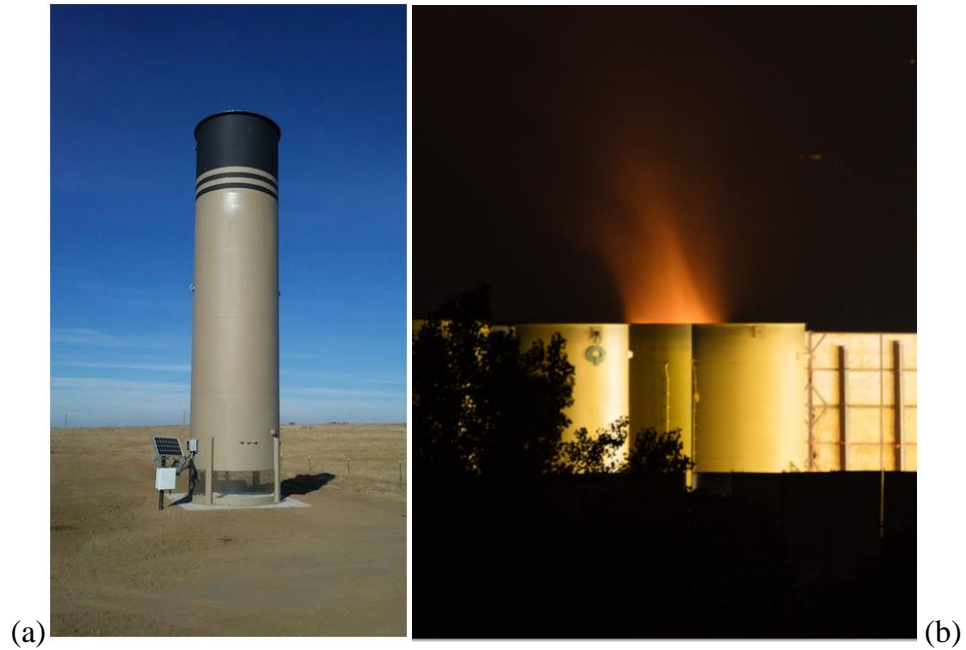
Figure 3. (a) Example of a combuster (Vapor Combustion Unit) used for burning gases during flowback. From https://gcollc.com/the-beast-3200 . (b) Combuster in night operation in Colorado.
