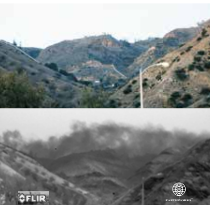
TOP: A clear afternoon in Porter Ranch, CA shows no sign of pollution from the nearby methane leak at the Aliso Canyon underground natural gas facility. BOTTOM: In the same location Earthworks' infrared camera reveals the air pollution that leaked for months, contributing 25% of California's daily methane emissions.
