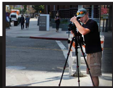
Pollution viewed with the naked eye versus an OGI camera, here coming from a manhole in a busy neighborhood in Los Angeles. The source is likely an abandoned oil well leaking underground.
