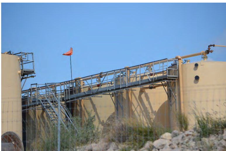
Figure 13. A windsock is often used at sites with H 2 S for workers to safely stay upwind of emissions.
