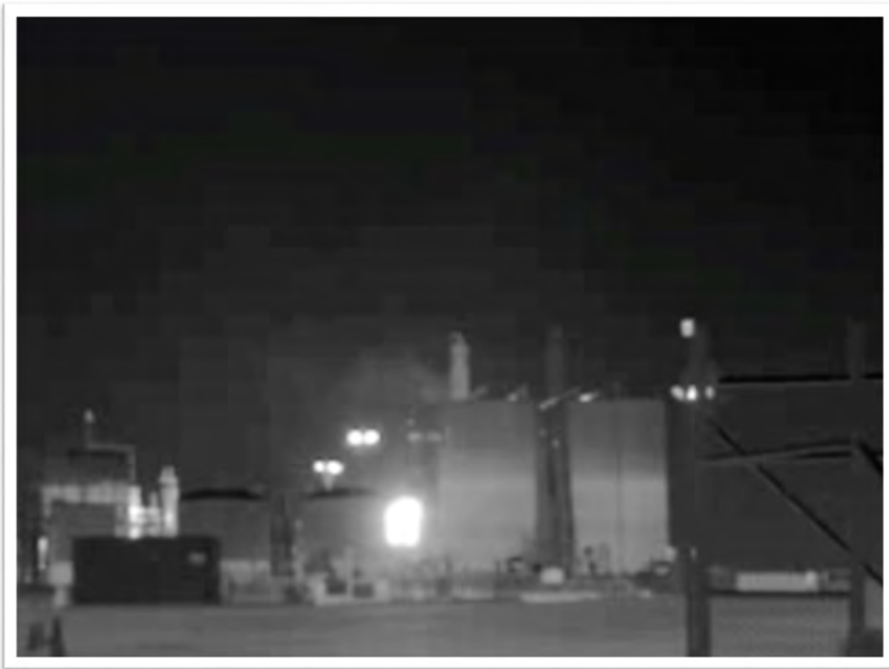
Figure 56. Still image of FLIR OGI video taken on March 7, 2014, showing Marathon Sugarhorn emission event that spiked a TCEQ air monitor 23 miles away. This emission event stretched over the course of three days, and during this time FLIR images were taken at Marathon Sugarhorn showing a plume emerging from equipment on site and travelling north towards Floresville. 162
