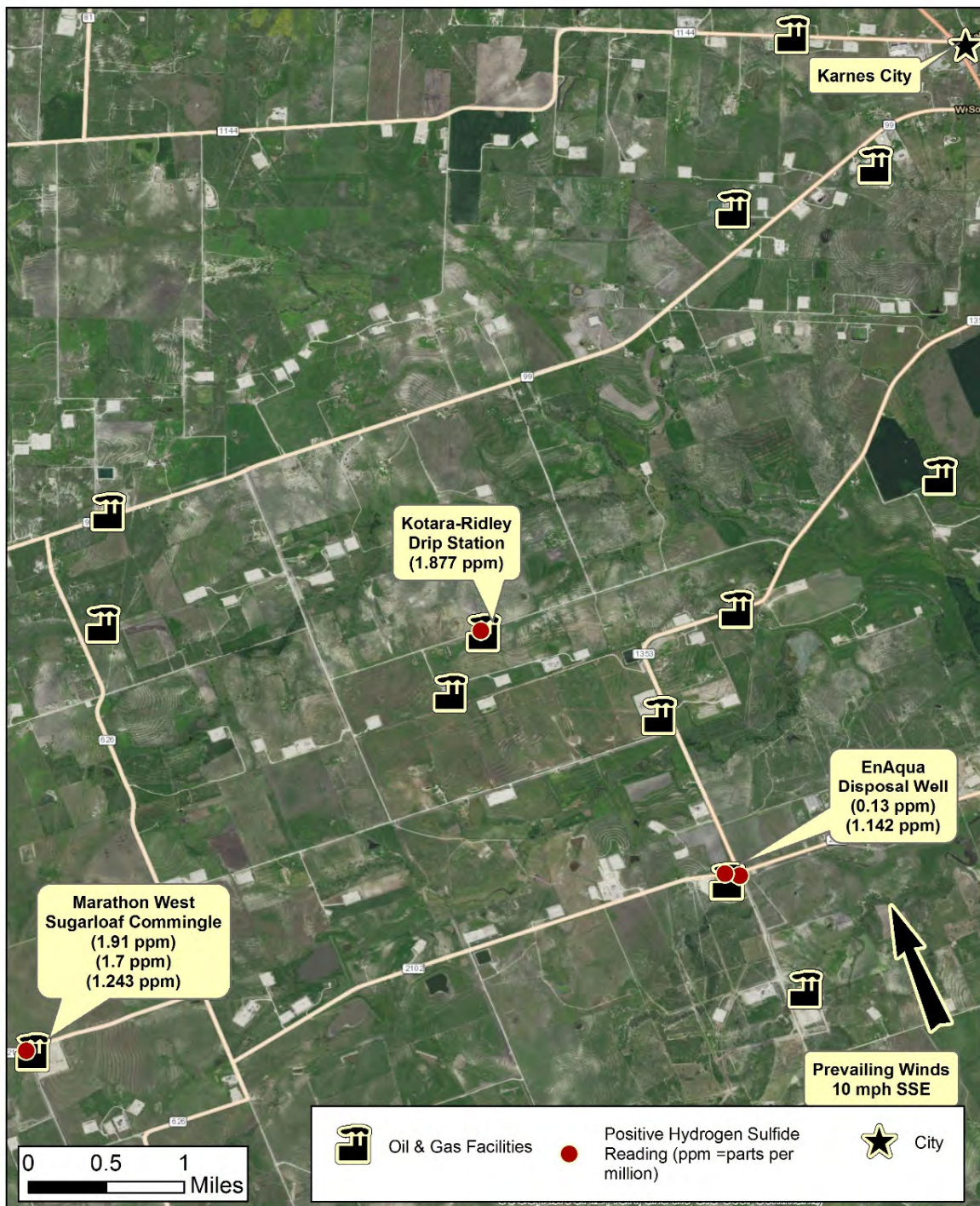
Figure 14. H 2 S levels detected with a Jerome Meter. Note: Jerome Readings were not necessarily taken at the same time as the SUMMA® samples.
