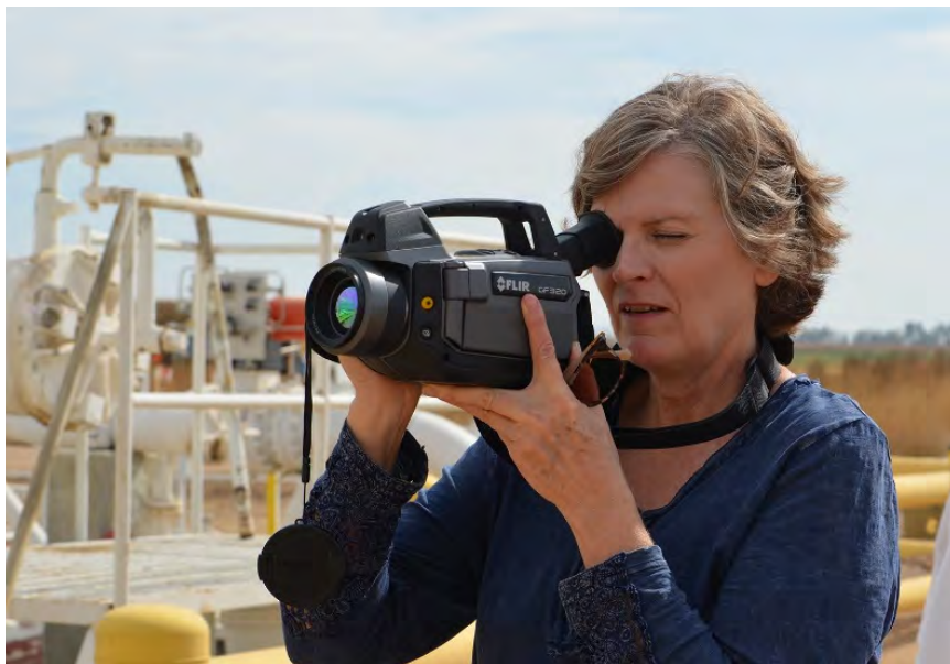
Figure 10, top: The FLIR Optical Gas Imaging camera (OGI) records infrared images of VOC emissions. At left shows the tanks as seen with the naked eye, and at right as seen with the OGI camera.
